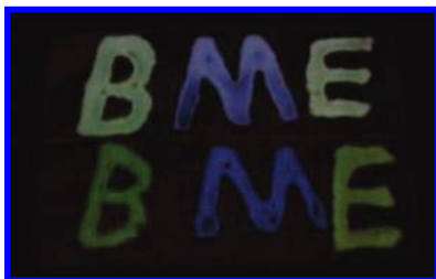
FIGURE 4. Photograph of colloidal crystal films composed of nigrosine-doped (bottom) and undoped spheres (top) with diameters of 220, 198, and 248 nm from left to right. These films were fabricated by drying the suspension at 60 °C.
